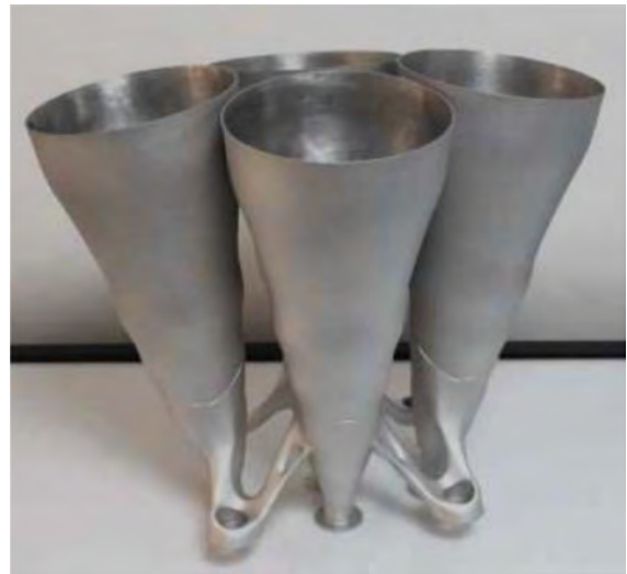
FIGURE 11. Ku-band spline horn cluster manufactured in aluminum using LPBF [65]. (©2018 Thales Alenia Space, printed by Volum-e, and developed in the frame of a CNES project).
